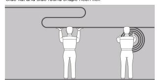
LED neon flex must be installed by at least 2 people, who can support the product in various locations as shown. During installation, care should be taken to ensure the bending radius of is not exceeded.
