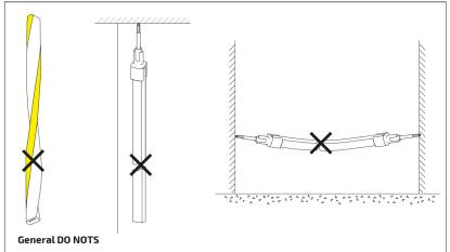
The images give indication as to what is NOT acceptable as an intended installation or during installation of other fixing methods
